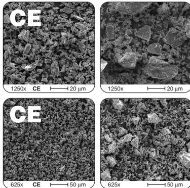
Particle size comparison of a colour in the CE series manufactured by Esmalglass-Itaca (left) with another commercial colour (right).
